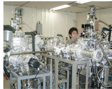
■超異種基板上的ヘテロエピタキシャル成長を実現するユニバーサル成長装置 Universal epitaxial chambers which make it possible to grow semiconductor films on various substrates with large lattice mismatches.
