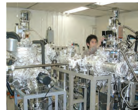
■ 超異種基板上のヘテロエピタキシャル成長を実現するユニバーサル成長装置 Universal epitaxial chambers which make it possible to grow semiconductor films on various substrates with large lattice mismatches.
