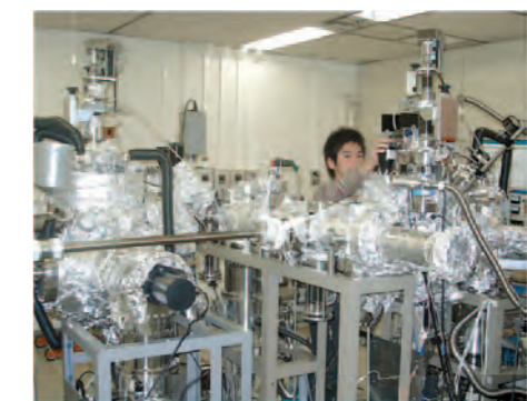
■ 超異種基板へのヘテロエピタキシャル成長を実現するユニバーサル成長装置 Universal epitaxial chambers which make it possible to grow semiconductor films on various substrates with large lattice mismatches.
