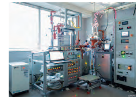
■ 熱制御用磁性複合材料の作製に用いる薄膜作製装置の例 Example of thin film fabrication equipment used to fabricate magnetic hybrid materials for thermal management
