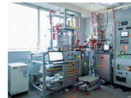
■ 熱制御用磁性複合材料の作製に用いる薄膜作製装置の例 Example of thin film fabrication equipment used to fabricate magnetic hybrid materials for thermal management
