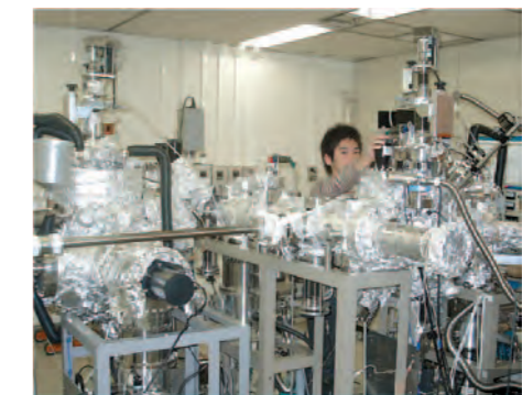
■ 超異種基板上的ヘテロエピタキシャル成長を実現するユニバーサル成長装置 Universal epitaxial chambers which make it possible to grow semiconductor films on various substrates with large lattice mismatches.
